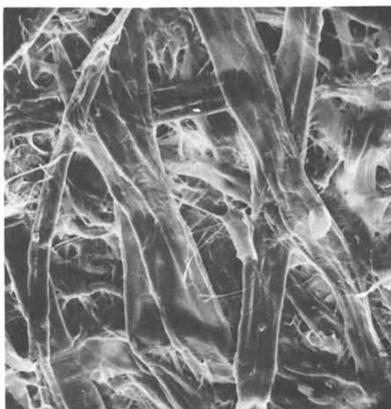
Figure 17. Scanning electron micrograph (255 \times ) of TMP handsheet: (a) untreated; (b) treated with 3% O 3
